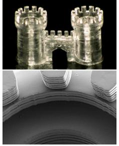
However, 3D printing usually creates parts with a rough surface along the printing direction due to the layer-by-layer based process (see Figure). In order to expand this process to the fabrication of optical components like e.g. lenses different surface finishing technologies for the reduction of the printed parts shall be evaluated.
